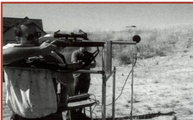
Mark Weiss demonstrates the correct position for testing sound levels on Gemtech's test frame. Note how the muzzle of the rifle is even with the microphone, on the same level, exactly 1 meter to the right of the microphone, per military specs.
