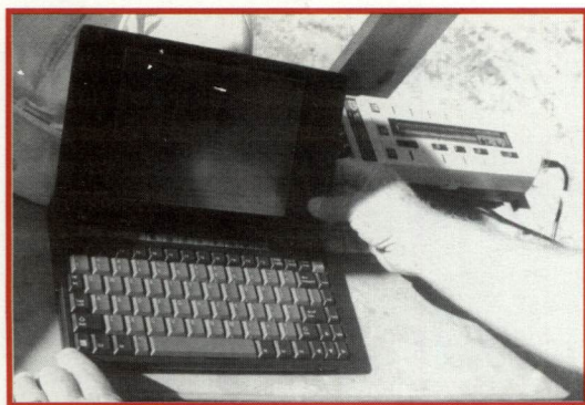
Phil Dater's custom testing setup. The Larson Davis 800-B meter on the right inputs to the HP Omnibook 425 computer with a special sound-based program written by Dater. Two of the reasons that the Omnibook 425 is used instead of a more modern laptop have to do with the LCD screen which is easily visible in sunlight—unlike most laptops, and the fact that it will operate for 7 or 8 hours using 4 AA batteries.
